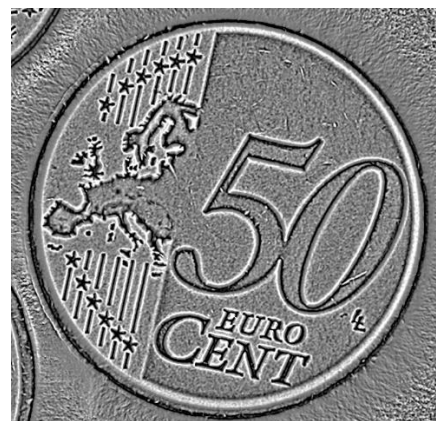
Figure 2 Topography (mean curvature) image of a 50 cents coin, taken from our sample images
